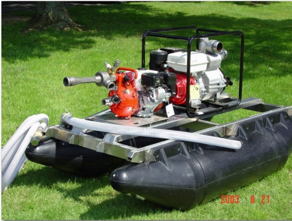
Figure 13: A portable hydraulic dredge may be necessary to remove accumulated sand from the channel.
